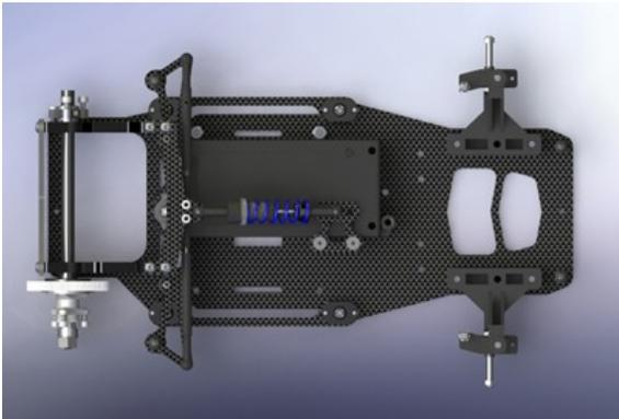
As you can see, the Rev 8 has been designed to allow for many different configurations. This allows the racer to choose the electronics they desire, and balance the chassis for best possible performance.
