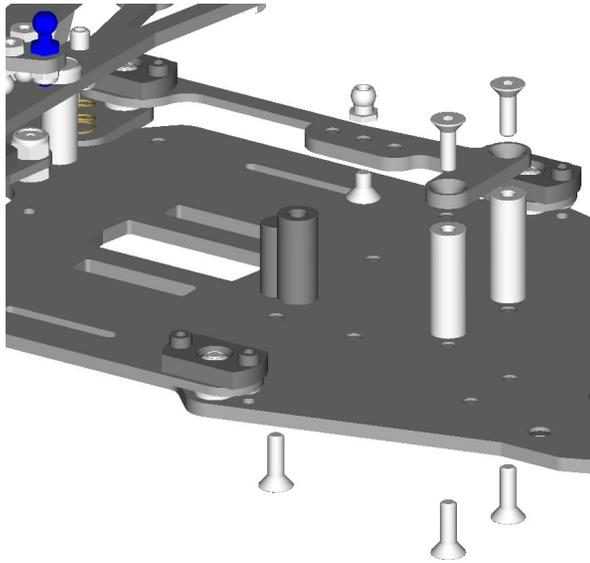
There are two different shock mounting plates included in the kit. This manual shows one configuration. Use the configuration that best suits your needs.
