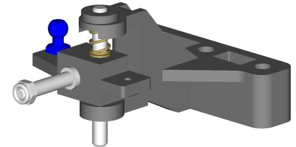
For the lower e-clip, using a pair of needle nose pliers, slide the e-clip with the open end first between the lower edge of the knuckle. Pinch the knuckle and lower arm to hold the e-clip in place. Use the back edge of a hobby knife blade to drive the e-clip in the rest of the way while keeping gentle pressure on the knuckle and lower arm.
