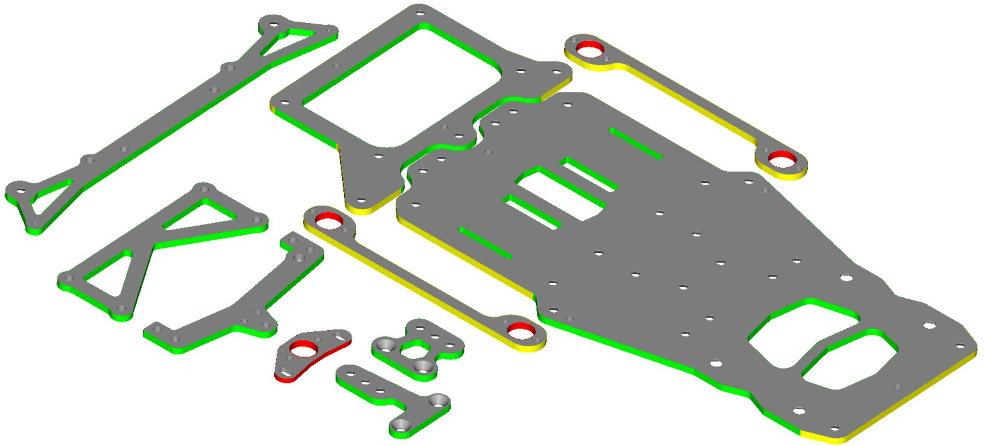
Some people like to sand/seal the chassis and other carbon fiber components with superglue for performance and feel. Do not sand or seal the areas shown highlighted in red. The chassis and rear pod plate areas highlighted in yellow are key areas for measuring the chassis. Care should be taken not to have glue extend below the chassis, as this could affect ride height measurement. Other components highlighted in yellow should not be rounded, only sealed, as this could effect strength.
