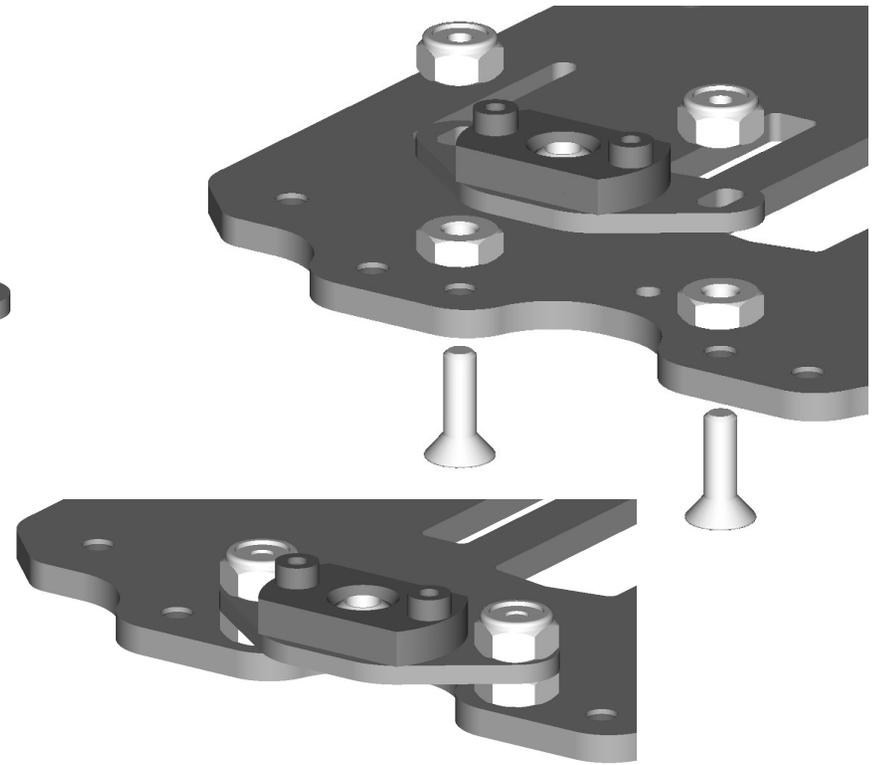
Attach the center pivot to the main chassis, leave the lower nuts loose until the pivot is installed onto the screws. Use needle nose pliers to hold the lower nuts in place while tightening the screws. Then install locking nuts.
