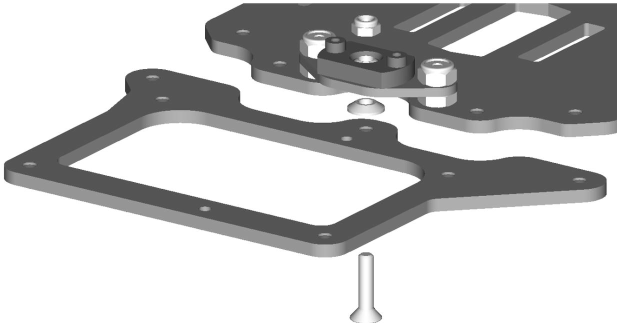
Thread the screw into the lower pod plate, low roll center cone, into the pivot ball first. This screw needs to be tight, be careful not to break your wrench or strip the hex in the screw. After the pod plate is attached, then install the locking nut.
