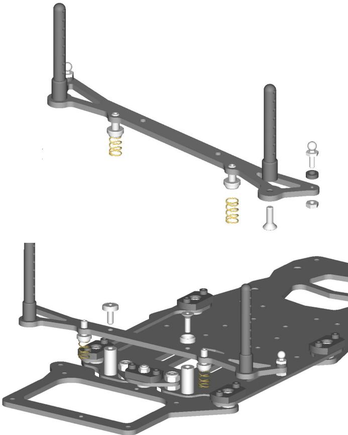
When the superglue has cured, assemble the tweak plate as shown: Attach the linear rate springs to the carriers. Install the 2-56 ball stud with spacers as shown. Attach the body mounts to tweak plate as shown. Attach stand-offs to the main chassis plate as shown (right).
