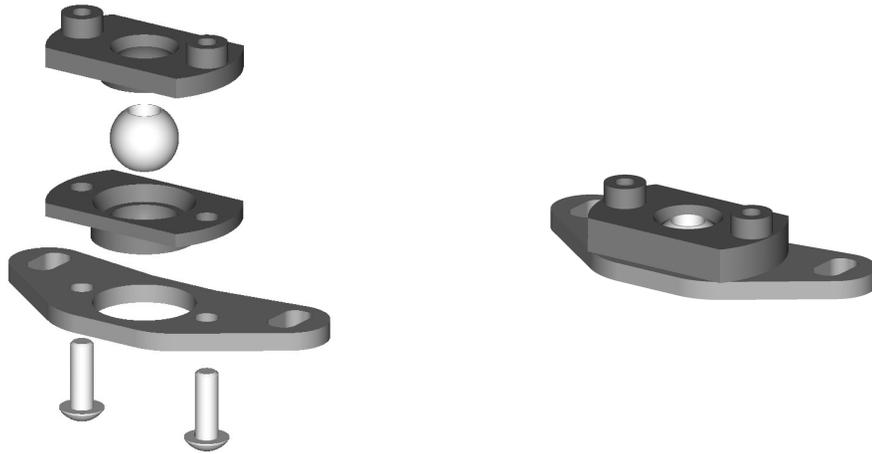
Assemble the center pivot as shown. Do not over-tighten the 2-56 button head screws. Find a 4-40 screw from the kit, and partially screw it into the ball. Use this screw to pivot the ball to judge how much to tighten the 2-56 screws. The ball should not have play in the socket, and it should not be overly tight. There are access holes in the chassis to adjust the 2-56 screws as they seat.
