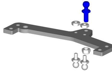
Pre-assemble the top plate with the 2-56 ball studs, then the 4-40 ball stud and spacer. Note orientation in the above drawing. Next attach the top plate with button head screws.
