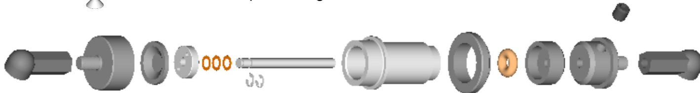
To assemble the main shock (damper):
