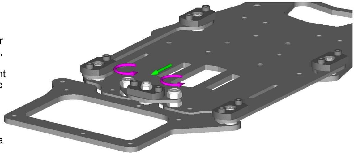
Screw the 6-32 set-screws through the tweak plate so that the wrench side is flush with the top of the tweak plate (the bottom of the tweak plate has counter sunk holes for the body mounts)
