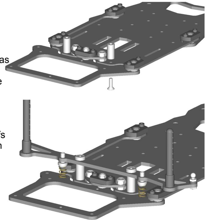
The aluminum bulkheads attach to the lower plate, then the rear plate to the bulkheads, all using flat head screws.
