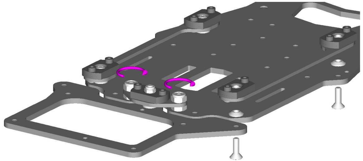
Assemble side links as shown above. Do not over-tighten the 2-56 button head screws. Find a 4-40 screw from the kit, and partially screw it into the ball. Use this screw to judge how much to tighten the 2-56 screws. The ball should not have play in the socket, and it should not be overly tight. There are access holes in the chassis to adjust the 2-56 screws as they seat.
