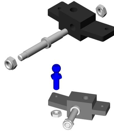
Push straight knurled side of front axle through the knuckle. Be sure to note direction of the knuckle. Use a thin flat nut to secure axle to knuckle.
