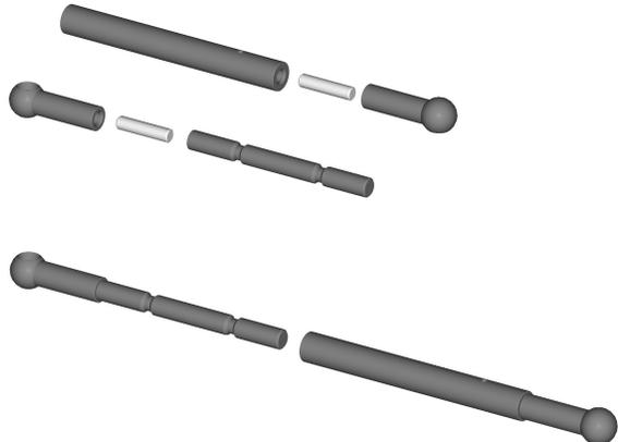
Assemble damper tubes as shown. Only screw the set-screw in half-way.
